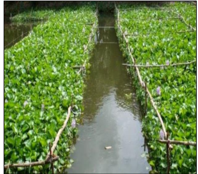
Fig 2 Water Hyacinth in a Controlled Environment for Wastewater Treatment Experiment and Removal of Excess Nutrient (Ratchanon Keawmanee, 2015).
